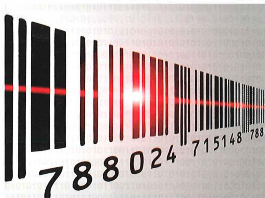
Figure 6.02 Light beams and light sensors are used to read barcodes
